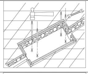
Mark out the fixing positions on the flooring basing on the body and drill four holes. Fix the floor screws into the holes.
